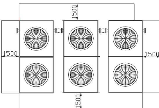
5) If there are wall around unit, the all should not higher than unit, and leave 2.4m from the wall. Leave 3-3.5m or above on the top, in case of air return.
