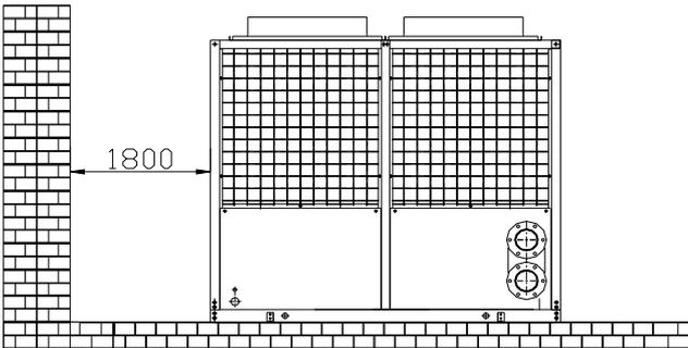
7) Add rubber dampers of 10-20mm between the unit and base.
