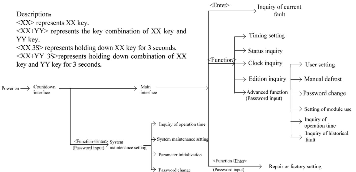
Note: 1. in branch interface (excluded count down interface and main interface), if no key action within one minute, the system will return to the main interface automatically.
