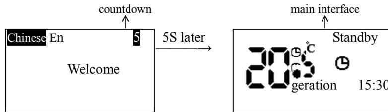
The above interface is normal starting-up interface of the unit when there is no fault. If other interfaces appear when starting up, please refer to [8. Troubleshooting](#)
