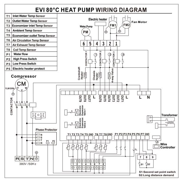
Note: crank heaters marked in diagram are optional parts according to customer request!
