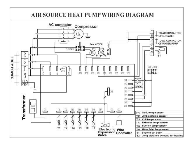
Note: 1. crank heaters marked in diagram are optional parts according to customer request!
